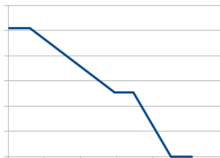
SP### very special : minimum & maximum values, center offset, output reversed enlarged neutral zone \pm 5\%
