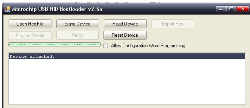
6. Open a new firmware, according to the version you want, with the button « Open Hex File »
